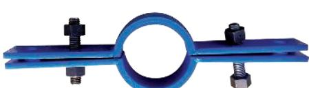
**STEEL CLAMP** to hold up the pipes during descent phase, to avoid thread buckling the clamp must be put at least at 300 mm distance from the pipe socket.
