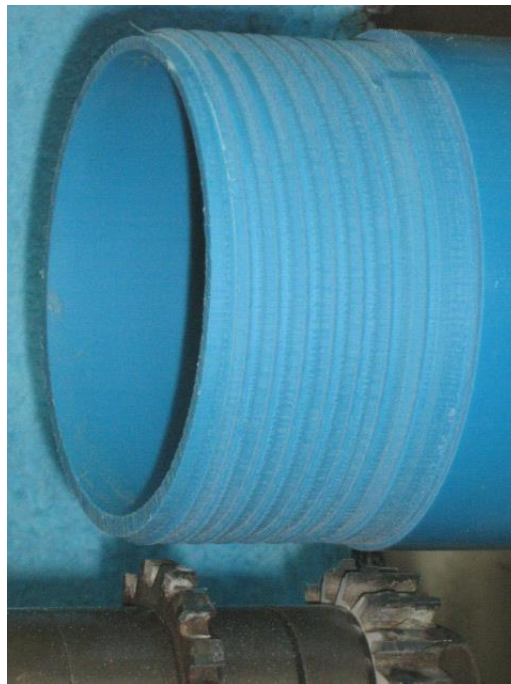
Pic. 2 Flush joints. This kind of connection requires the same overall dimensions as the pipe diameter.
