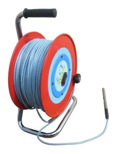
Portable water level probe for water table measurement in water wells, piezometer wells etc... This instrument consist in a round measurement cable, available in various lengths from 10 m to 500 m, with 304 stainless steel ferrule 12 mm. The probe is also equipped with cable winding device, handle for transport and printed circuit board with buzzer, warning light and flat battery led.
