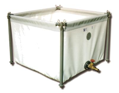
Flexible tank to contain liquids, made of extrastrong polyester fabric coated with plastomer, supported by an easily assemble metal frame. Volume from 1 m<sup>3</sup> to 60 m<sup>3</sup> (depends on the tank dimensions, see chart below). When unused the tank can be refold and reduced to a minimum size.
