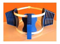
Plastic centralizer to keep the column in a central position during the phase of descent. Is composed of three clamps with fins to make it adaptable to different diameters of the perforation. The fins, equidistant between them, can be cut to fit the required dimensions.
